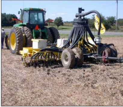
Figure 5. For the most effective application, liquid manure should be applied shallow and uniformly into the soil surface. (Photo courtesy of Jon Rausch, The Ohio State University).
